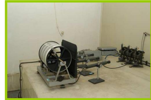
**Electromagnet seismometer with galvanometric registration**
