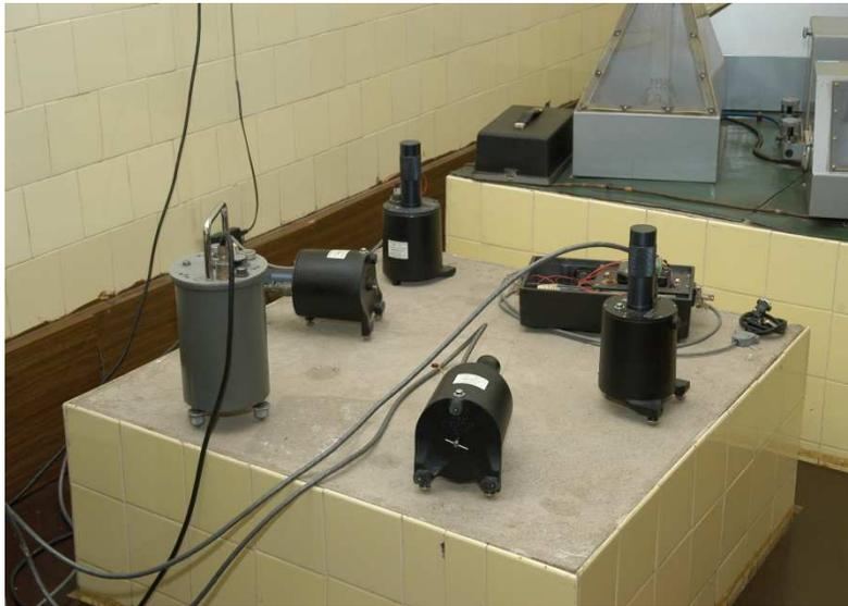
**electromagnetic seismometers SS-1 (short-period) and WR-1 (wide-range period)**
