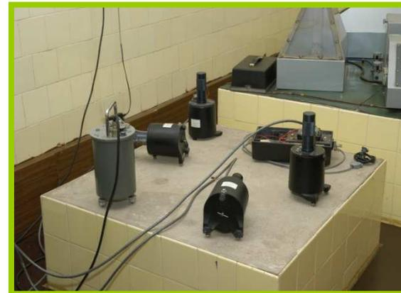
**Electromagnetic seismometer with digital registration with SSR-1**
